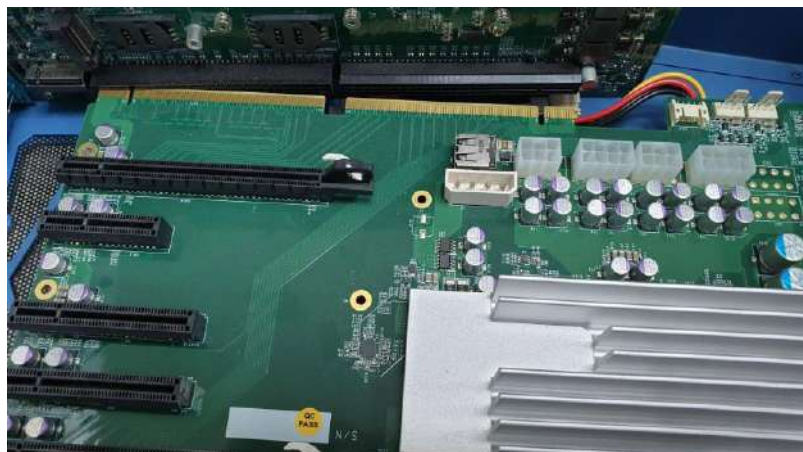
Disengage the daughter-board from the motherboard
