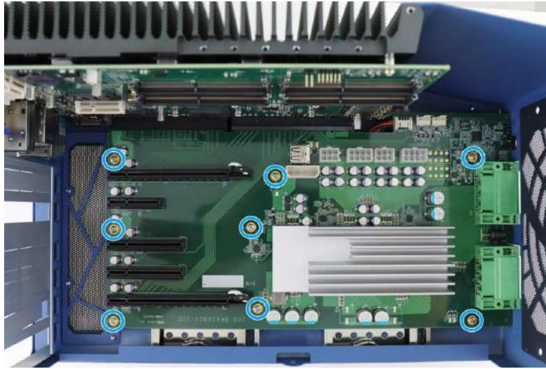
Remove screws securing the daughter-board
