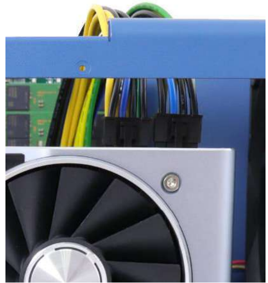
6 or 8-pin power connector on graphics card
